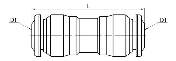
**MATERIAL:** NICKEL PLATED BRASS BODY. TECHNOPOLYMER RING.
